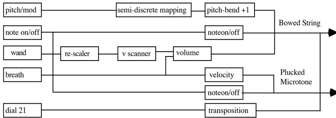
[fig.5 LightHarp Control Modes for Microtonality]
